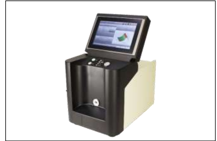
Elipsometer for fuel quality
