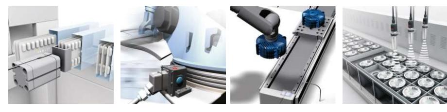
Magnetic sensors monitor the position of pneumatic grippers in the packaging industry. Mechanical sensors are ideal for position detection in robotics control.
