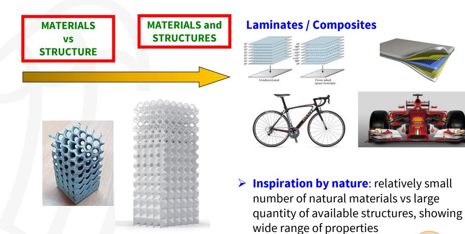
Architectured materials: combinations of two or more materials, or one material and space (pores), designed to display attributes not offered by one material alone
