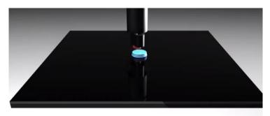
**FDM** (*Fused Deposition Modeling*) uses a thermo-plastic filament, pushed through a heating chamber and extruded through a small nozzle
