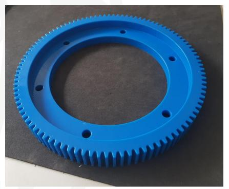
Original component in reinforced plastic was turned into an AM component realized with PolyJet technology in a photo-polymeric resin
