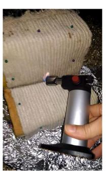
Flame test on "Cannettone ciniglia" fabric with mixed resin
