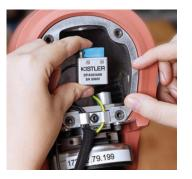
Pressure sensors for combustion measurement, together with amplifiers and indicating cycle analyzer, allows engineers to gather precious data and develop cleaner, efficient engines for future mobility
