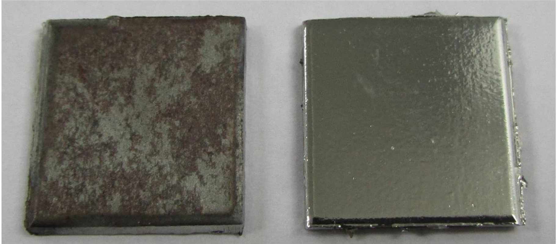
Stainless steel coating onto carbon steel
